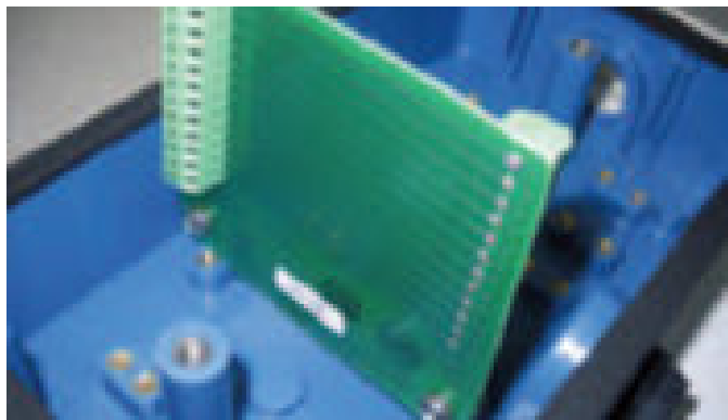
Figure 19: Junction Box PN 23550-00 has an Extension Board but no Preamplifier
