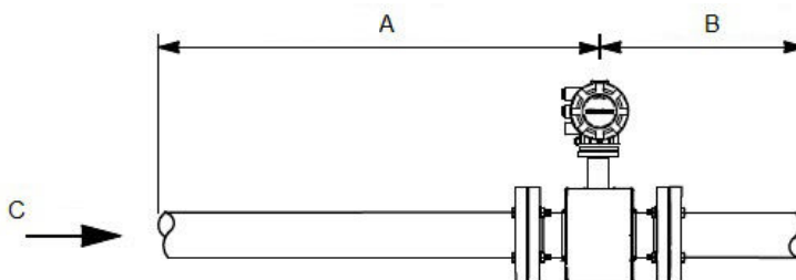
Figure 3-2: Upstream and Downstream Straight Pipe Diameters
